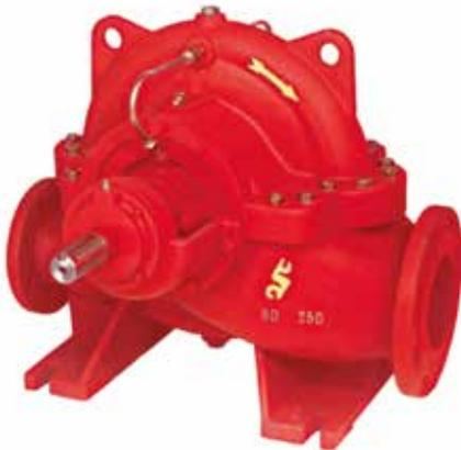
Horizontal, single stage, axially split volute casing pumps with double suction radial impellers.
