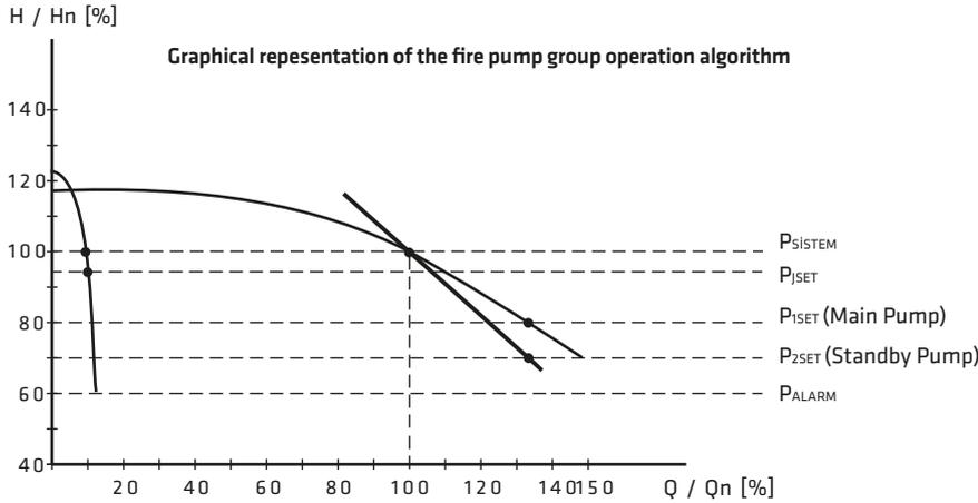
If the pressure drops below the set value ( $P_{JSET}$ ), jockey pump starts running with the signal coming from the pressure switch and continues to run for 10 minutes until the system pressure reaches the set value ( $P_{SYSTEM}$ ). If the pressure continues to drop, ( $P_{ISET}$ ) first the main pump starts to run. If the system pressure ( $P_{SYSTEM}$ ) can not supplied and pressure continues the drop
